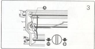
Adjust the oil amount of the rotating hook by turning the oil amount adjusting screw (A). Turn the screw(A) clockwise (in the "+" direction) to increase the oil amount; turn it counter -clockwise (in the "-" direction) to decrease the oil amount.
