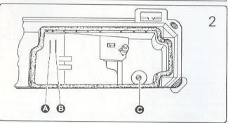
1). The oil amount in the oil reservoir is controlled through the reference marks A and B shown in Fig. 2 The mark A indicates the max. oil amount level, the mark B for the min. oil amount level. If the oil amount level is under the mark B, replenish the oil reservoir with oil in time.
