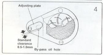
In ordinary operation, adjustment is not required for the oil pump. If oil splashing does not occur in the oil check window when the machine runs at a low speed (approx. 2000 spm), close the clearance of the bypass oil hole.
