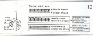
Thread tension should be determined in accordance with the stitches obtained by adjusting the tension of the bobbin thread and needle tension (Fig. 12).
