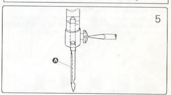
Turning the balance wheel to lift the needle bar to the upper end of its stroke. Loosen the needle clamp screw while keeping the long groove of the needle leftward, fully insert the needle shank up to the bottom of the needle socket, then tighten the needle clamp screw.
