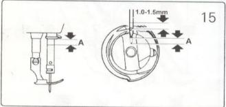
When lifting the needle bar from its lowest position of the stroke to the distance A, the hook point D of the bobbin should align with the center line of the needle and be 1.0 – 1.5 mm above the upper end of the needle eye. (Fig. 15)
