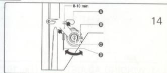
The tension of the needle thread: to be adjusted by turning the thumb nut.
