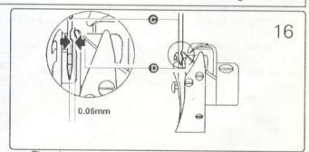
The clearence between the bottom of the needle notch and the hook point should be 0.05 mm(Fig. 16).
